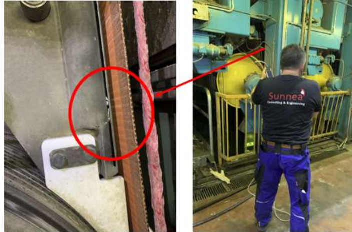
Figure 8. Regular maintenance of runnability components (findings: depositions of dirty in blowing slots)
